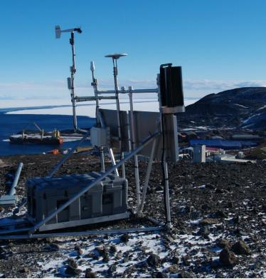
Our LE-v50 Extreme vertical axis turbine is specially adapted for storm force winds and sub-zero temperatures. The LE-v50 Extreme will trickle charge your batteries or provide energy for low power electronic devices such as data-logging and telemetry equipment.
